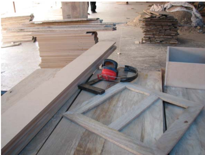
The planks are sorted and stacked according to their sizes and quality.
